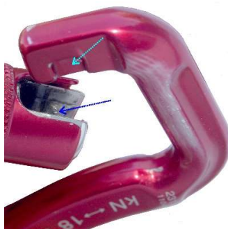
Photo n°9 : Half-detail of the locking groove and locking lug
