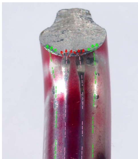
Photo n°3 : Direct positional correspondence between the fracture initiation areas and the longitudinal protrusions on the supporting working surface of the carabiner
