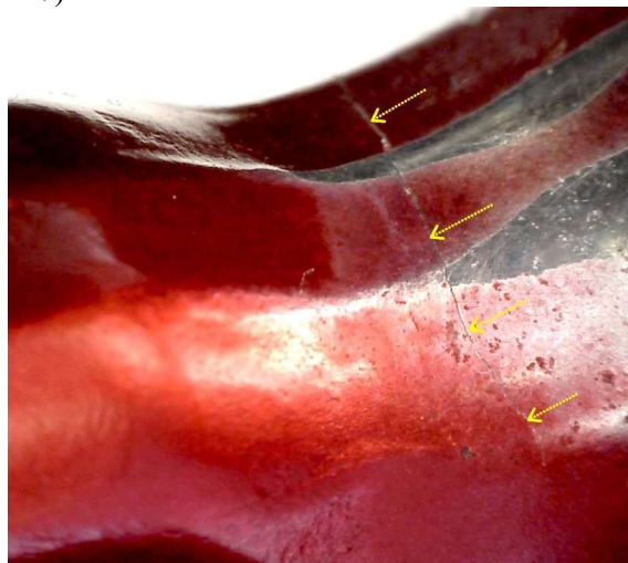
Photo n°6 : The beginning of fatigue fracture on carabiner n°2 in exactly the same places where it was initiated in the case of carabiner n°1
