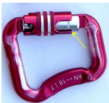
Photo n°8 : Carabiner n°2 and marked side of the locking mechanism where the grooves and protrusion are located
