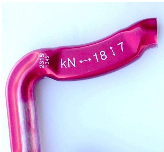
Photo n°7 : Static loads declared by the carabiner manufacturer in the longitudinal and transverse direction
